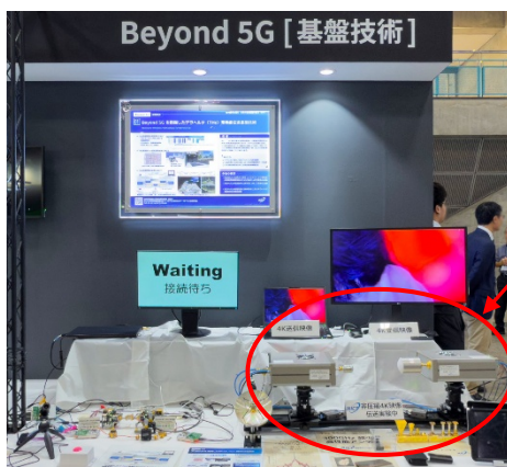
[fundamental technology] Demonstration of uncompressed 4K video transmission system using 300 GHz-band terahertz waves
