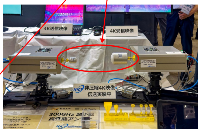
[fundamental technology] Demonstration of uncompressed 4K video transmission system using 300 GHz-band terahertz waves
