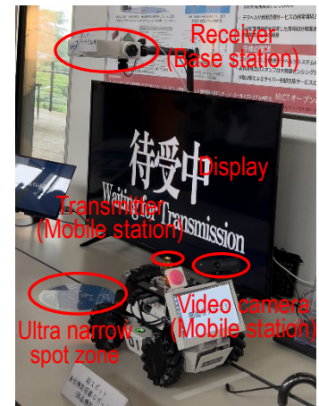
Fig. 2 Ultra Narrow Spot Wireless Service Demonstration System
