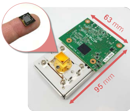
Fig. 3 IEEE802.15.3e Compliant Millimeter Wave Wireless Communication Module and Main Specifications
